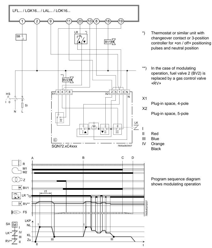
No. A Number of internal diagram (second position after the dot in the type reference)
