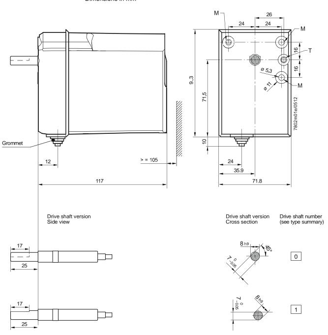
All drive shafts shown in end switch position II «Closed» as supplied.
