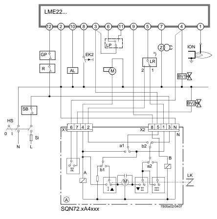
Thermostat or similar unit with changeover contact (2-wire control), or 3-position controller for «on / off» positioning pulses and neutral position
